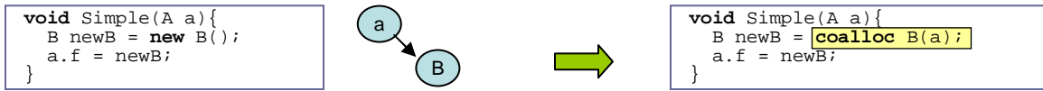
Figure 2: Simple example: the newly allocated B object is stored in the A object parameter, therefore we convert the new into a call to coalloc, passing a as the colocator.
